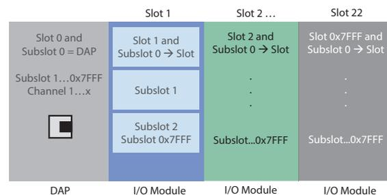
Figure 5: Addressing of I/O data in PROFINET on the basis of slots and subslots
