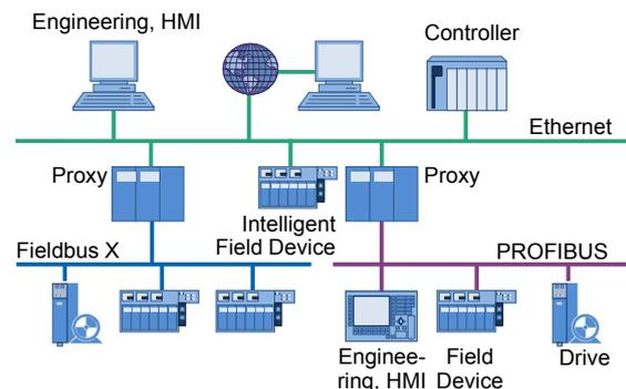
Figure 25: Integration of fieldbus systems is easy with PROFINET
