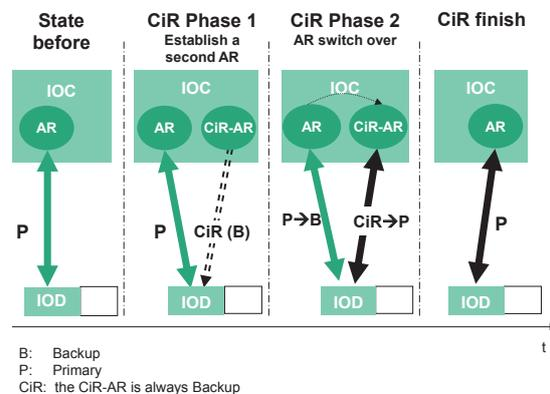
Figure 23: Configuration changes without plant interruption thanks to redundant connection
