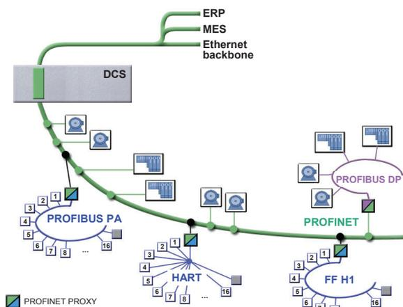
Figure 26: Example architecture for use of PROFINET in process automation
