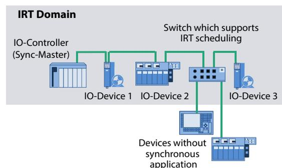
Figure 18: Mixed operation of synchronized and unsynchronized applications
