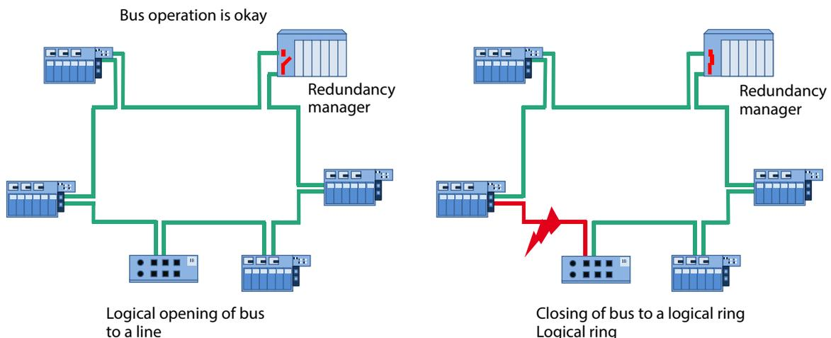
Figure 24: Preventing circulation of frames by logical separation of the bus
