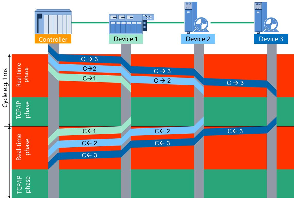
Figure 17: IRT communication divides the bus cycle into a reserved interval (red) and an open interval (green)
