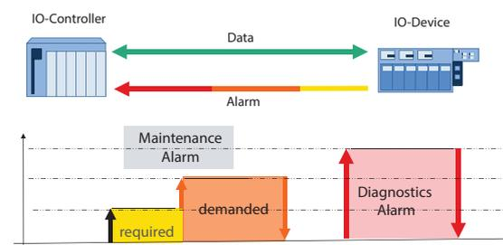
Figure 11: Diagnostic model for signaling faults with different priority
