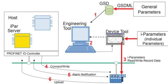
Figure 22: A parameter server can be used to automatically reload backed-up data during device replacement
