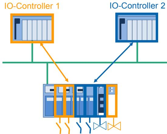
Figure 20: Shared device: Access by multiple controllers to different modules in a device
