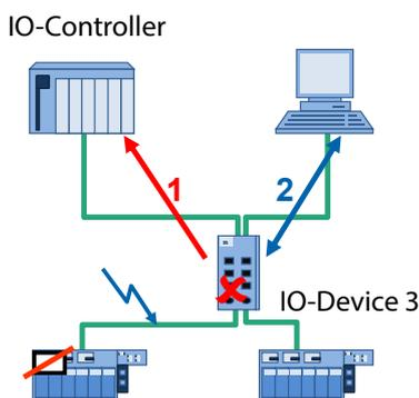
Figure 15: Integration of network diagnostics into the IO system diagnostics
