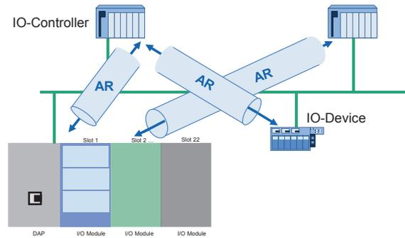
Figure 7: A field device can be accessed by multiple application relations
