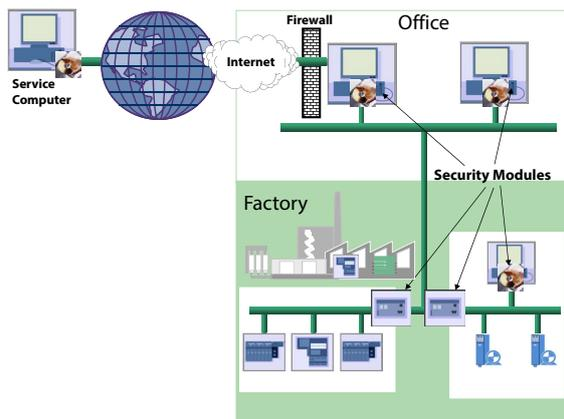
Figure 29: Access to machines and systems using secure connections
