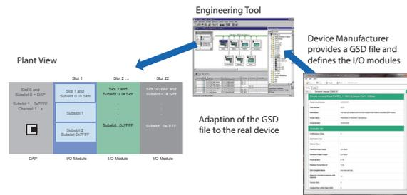
Figure 9: Assignment of definitions in the GSD file to IO devices when configuring the system
