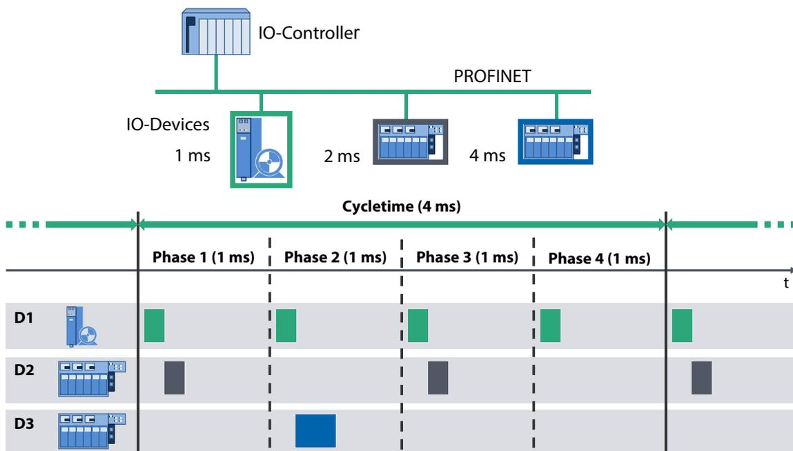
Figure 10: Real-time communication with cycle time monitoring
