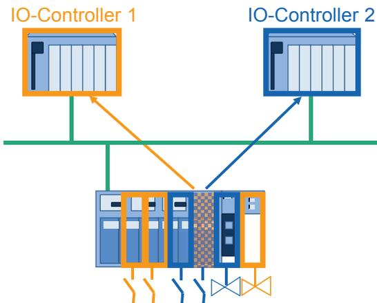
Figure 21: Shared input: Multiple controllers read the same inputs on a device
