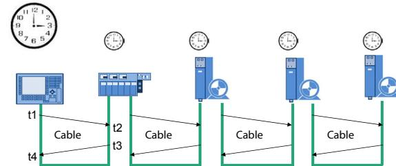
Figure 16: Synchronization of clock pulse generators within an IRT domain by the clock master
