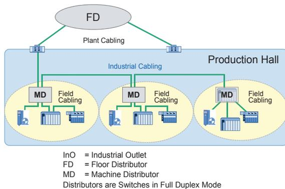
Figure 27: Ethernet networks in industrial environments usually have line topology
