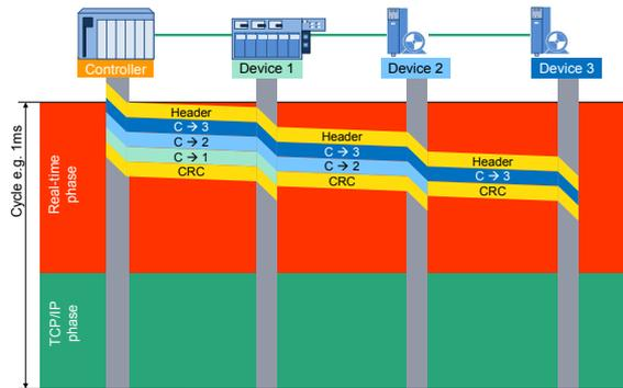
Figure 19: Packing of individual frames into a group frame
